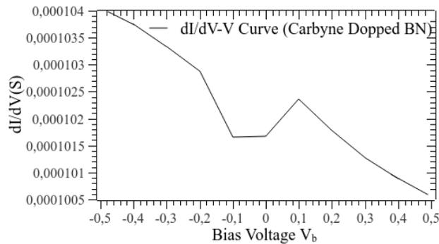
Fig. 3. Differential conductance versus voltage curve for Carbyne doped with B and N.
