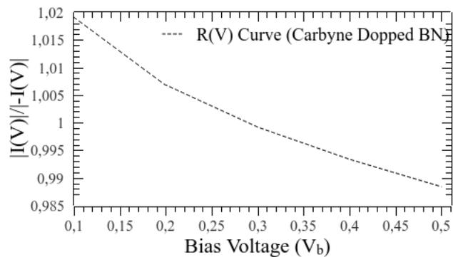
Fig. 4. Rectification ratio curve for carbyne doped by B and N.
