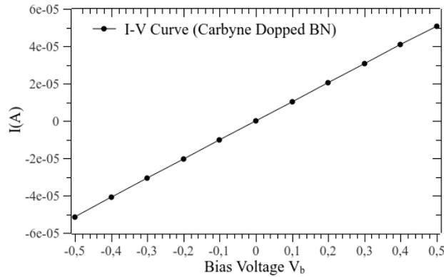
Fig. 2. Voltage versus current curve for carbyne doped with B and N.
